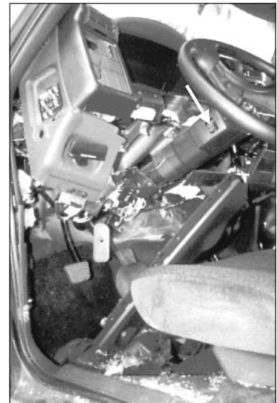
Figure 7. Truck interior. Wheel column is separated from its attachment to the instrument panel and the socket for wiper-control stalk (arrow).
